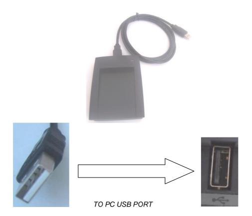
When pluging the YHY101U reader to the PC's USB port, the system will recognize it as a HID keyboard device.
