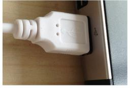
When plug the ER300L reader to the PC's USB port, the system will recognize it as HID keyboard device.
